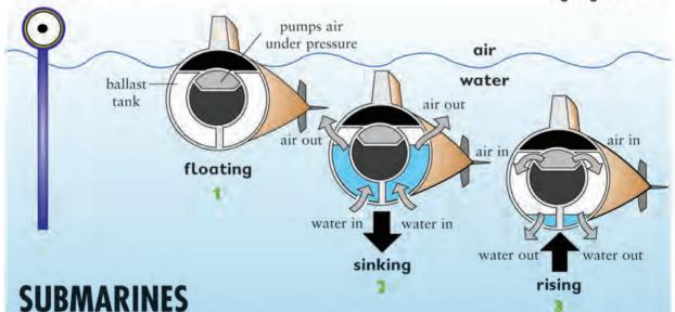
Submarines are ships which can float and also sink. They have cigar-shaped hulls and a conning tower on top. They are able to travel to the depths of the ocean as well as sailing on the surface. Because of this, the hull must be strong enough to withstand great pressure. Submarines are able to float and sink because they contain large ballast tanks. Pumps on the submarine adjust the amount of air or water in the tanks. When the submarine floats, the ballast tanks are full of air.
